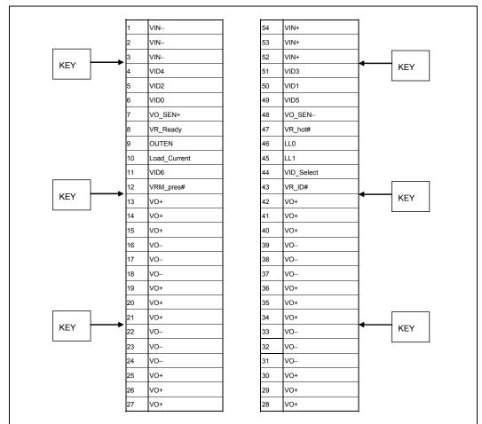
Figure 7-1. VRM 11.0 Pin Assignments
